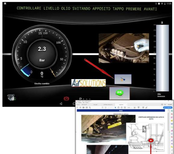
If necessary, add oil by pressing the DROP button to start topping up the oil
