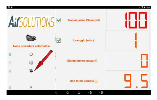
Once the operation is finished, by pressing the print button it is possible to print the report of all the operations carried out
