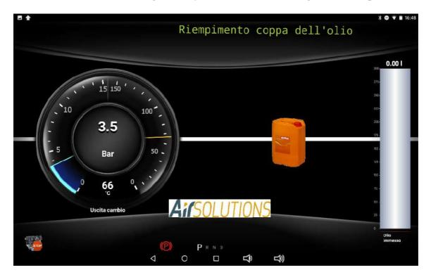
ATM09.18 will then fill the previously assembled sump with new oil. If in the first screen of the "automatic procedure start" the cup filling field had not been filled, the ATM09.18 in this section will propose as the quantity to be entered the same quantity of the oil that it has discharged. Only in this case increase by pressing the + button the quantity of oil to be added by adding any residual quantity of oil left in the cup during the disassembly operation
