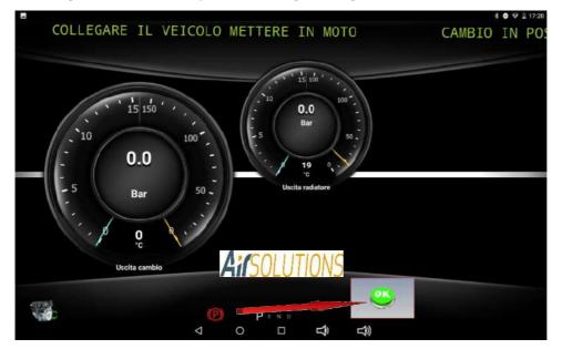
after starting the engine (if required) press the "OK" button and visually check the level according to the procedure indicated in the file downloadable from the database using the appropriate button
