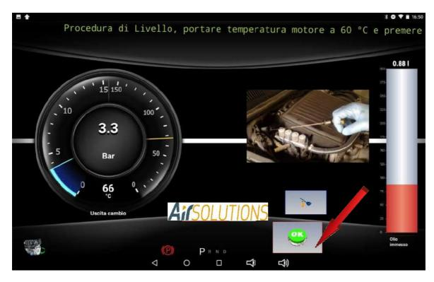
proceed to check the correct oil level by pressing the OK button
