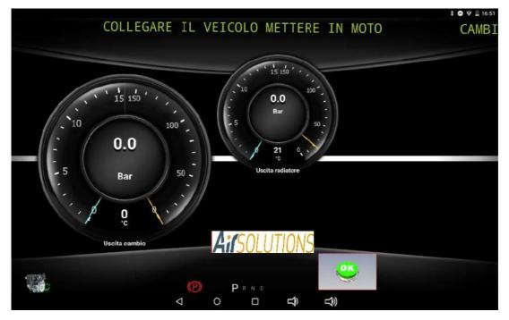
Press the OK button to detect the correct flow of oil. As soon as detected turn off the car
