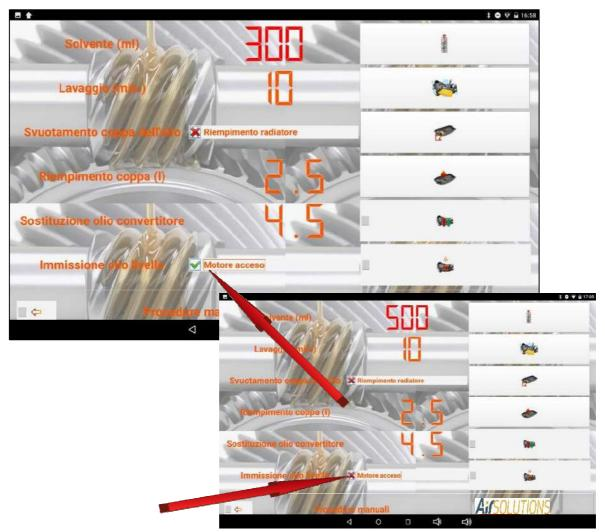
after connecting the ATF Smart ML pipes following the procedures shown in the database, start the engine as indicated by the scrolling message
