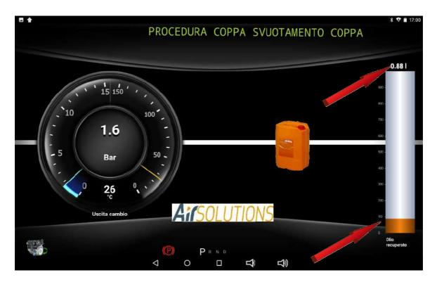
At the end of the cup emptying, the ATM will notify that it has completed the phase (if required by the type of transmission - otherwise this phase will be skipped and the procedure will automatically restart from the converter oil replacement procedure)
