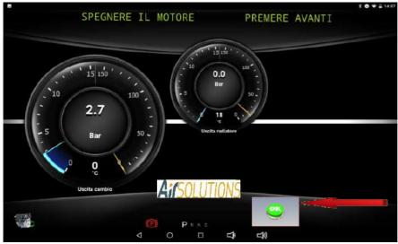
Once the correct direction of oil flow has been recognized, the ATF Smart ML request that the car engine be turned off by pressing the OK button
