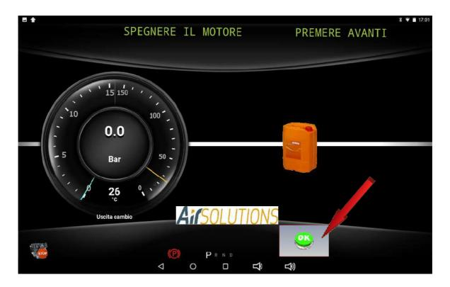
a container for collecting the used oil must be positioned under the sump (if required by the type of transmission - otherwise this phase will be skipped and the procedure will restart automatically from the converter oil replacement procedure) and after pressing the OK button
