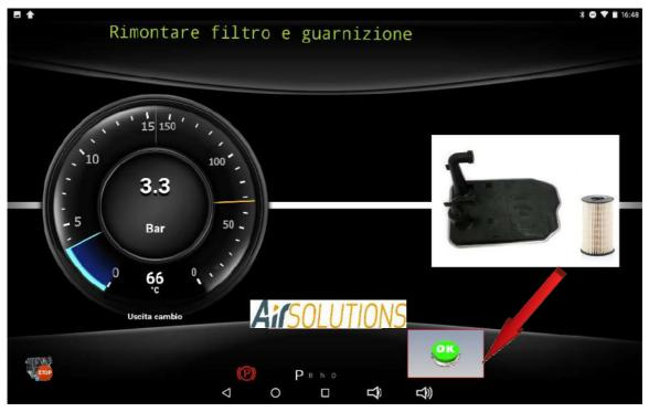
Press the OK button after having correctly reassembled the filter, gasket and cup
