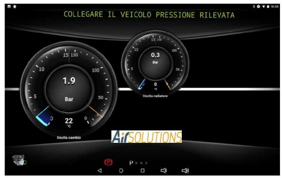
The ATF Smart ML checks the correct direction of oil flow by reading the input and output pressures of the gearbox
