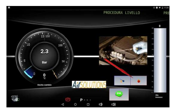
Once the correct oil level has been restored, press the DROP button again to finish the oil injection
