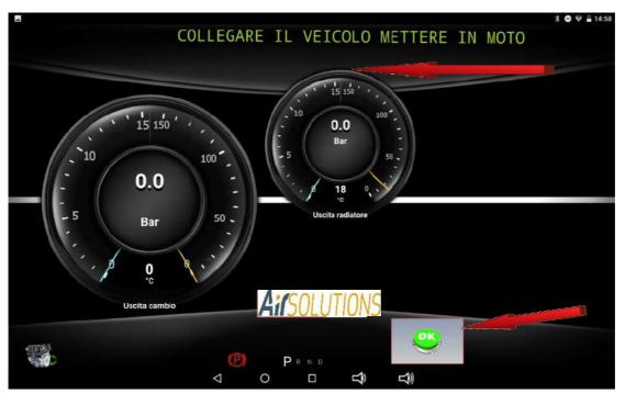
after starting the engine press the "OK" button and start the washing phase of the transmission. The residual washing time is highlighted
