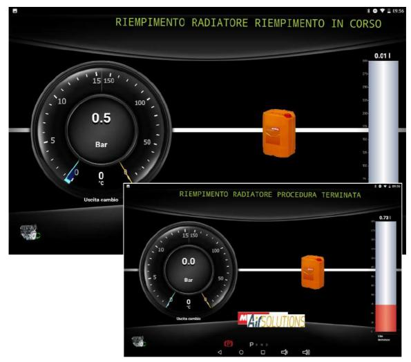
once the oil has been filled in, the ATF Smart ML will proceed to flush it into the cooling system, highlighting the passage of the set time in the clock
