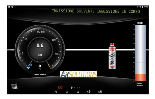
If checked on the solvent input operation, the ATF Smart ML will enter the set quantity At the end of the solvent input procedure, the automatic transmission washing procedure will automatically start for the duration previously indicated
