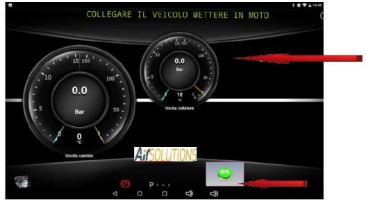
after starting the engine press the "OK" button, the ATF Smart ML will recognize the correct direction of oil flow
