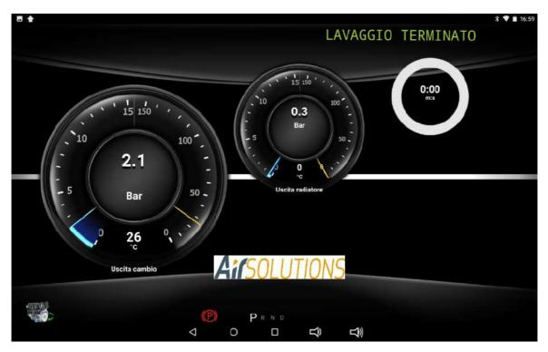
As the cup is emptied, the ATF Smart ML weighs the drained oil and the measured pressure will tend to drop towards zero (if required by the type of transmission - otherwise this phase will be skipped and the procedure will automatically restart from the replacement procedure converter oil)
