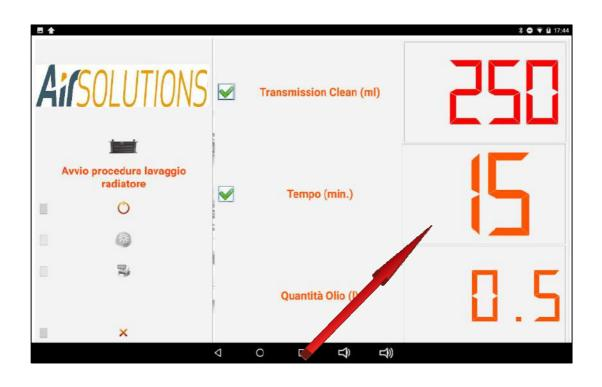
clicking on the Start procedure button will activate the washing cycle of the cooling system
