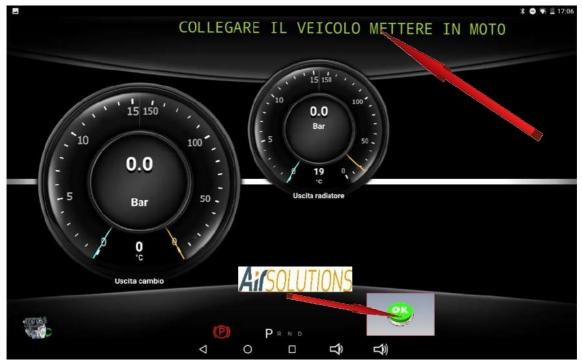
after starting the engine, press the "OK" button. The ATF Smart ML will begin to replace the oil inside the converter. The phase will be carried out by emptying 100 grams of used oil and introducing 100 grams of new oil at a time until the complete replacement of the quantity previously set
