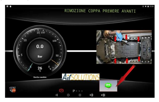
after removing the cup and the filter, press the OK button
