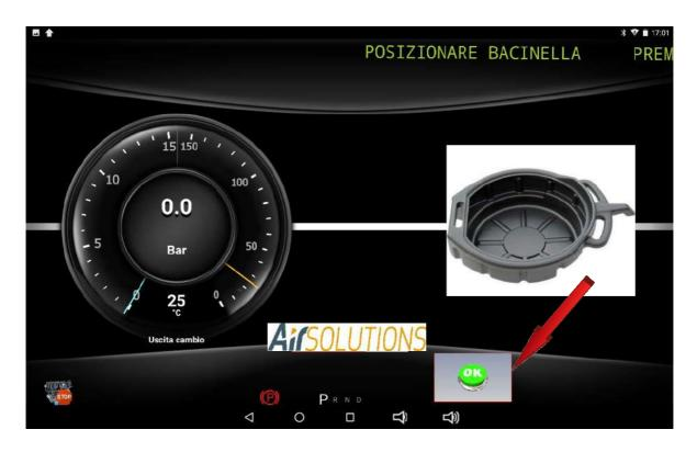
proceed with the removal of the sump paying attention to the fact that surely a small quantity of oil will remain inside the sump itself. Remove the sump, taking care not to spill the exhausted oil content (if required by the type of transmission - otherwise this phase will be skipped and the procedure will automatically restart from the converter oil replacement procedure) and press the OK button
