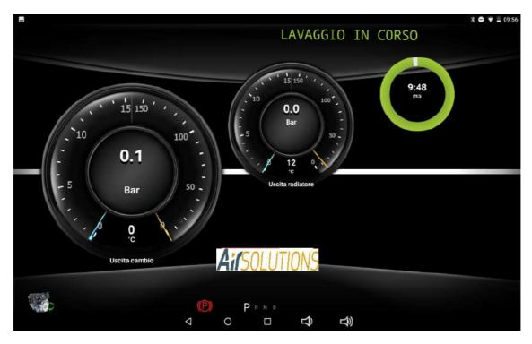
at the end of the washing, the ATF Smart ML recovers the used oil used for washing
