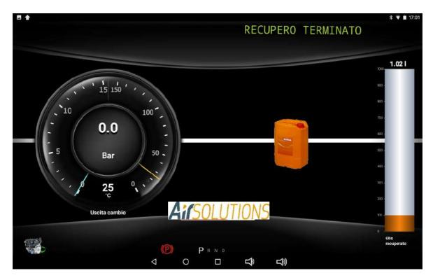
asking to stop the engine. After turning the engine off, press the OK button (if required by the type of transmission - otherwise this phase will be skipped and the procedure will automatically restart from the converter oil replacement procedure)
