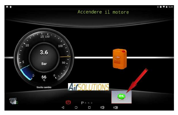
press the OK button after starting the engine
