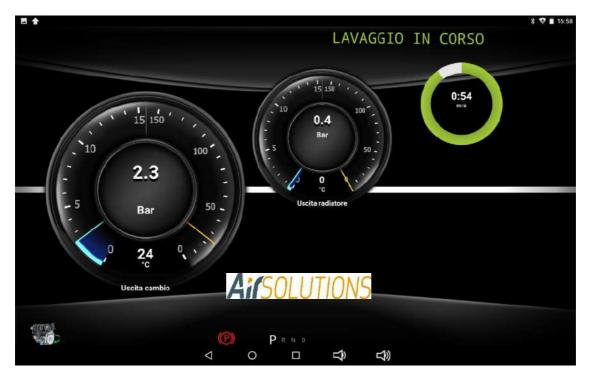
At the end of the automatic transmission washing procedure, the ATF Smart ML proceeds to empty the cup (if required by the type of transmission - otherwise this phase will be skipped and the procedure will automatically restart from the converter oil replacement procedure)
