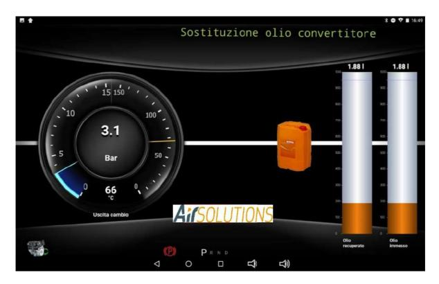
The ATF Smart ML will begin to replace the oil in the converter indicating the quantity of oil introduced and the quantity of oil recovered
