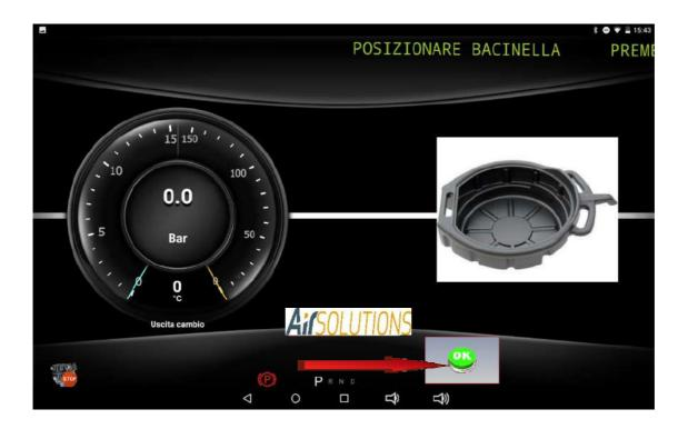
Place a container to collect the spent oil under the cup and then remove the cup
