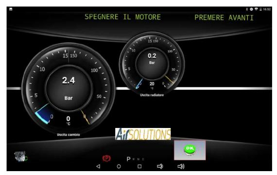
Act on the OK button. The ATF Smart ML will begin the cup filling procedure by highlighting the quantity gradually entered on the scroll bar
