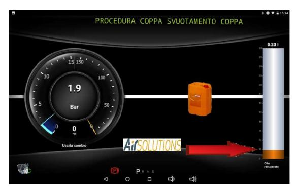
press the OK button, the ATF Smart ML will start to empty the automatic transmission cup
