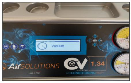
4) Make sure that the quick couplings are completely closed, then press the Ok button. The machine will start to carry out the vacuum procedure for 15 minutes
