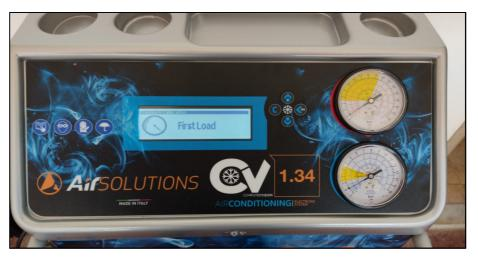
8) press the OK button. The machine will automatically draw 600 gr. of gas from the external cylinder. At the end it will stop autonomously and the display will indicate again the msg "first charge"
